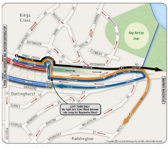
Figure 2.3 Traffic flow for Bayswater Road and the Ward Avenue ramp.
